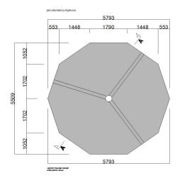
Edge-reinforced concrete slab
